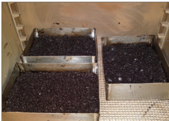
Fig. 2 loose mix in a flat pan placed into a Forced Draft Oven
